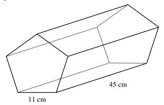
The cross section is a regular pentagon. The volume of the prism =  $9368 \text{ cm}^3$
